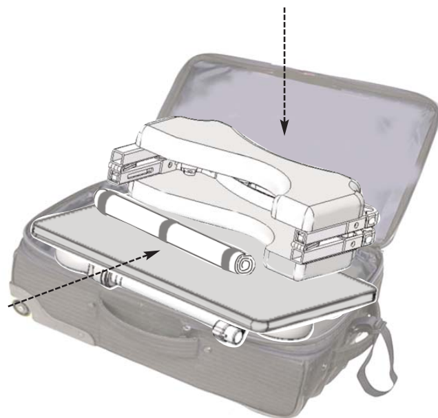
Figure B - Insert the rolled up cloth back in to the cavity of the seat frame. Then place the folded seat frame on top of the double side foam panel.
