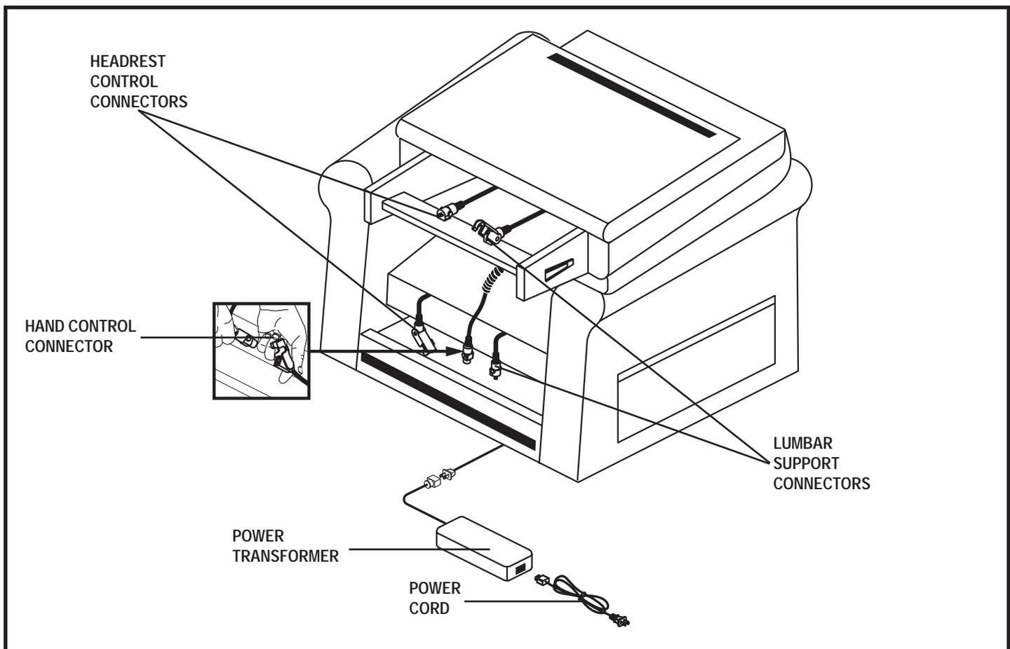
Figure 2. Chair Assembly - Power Transformer, Cords, and Connections
