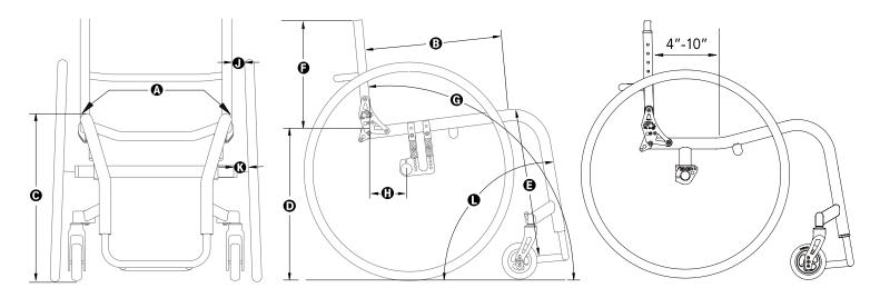
REAR SEAT WIDTH @ Measure from outside of seat tube at back post to the outside of the opposite seat tube at back post.
