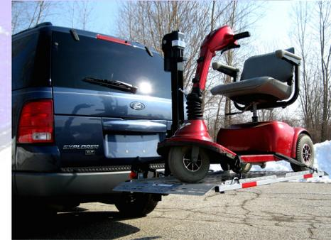
US208P has a pocket for Mid- Drive Mobility devices to rest in for secure travels.
