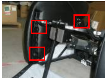
The position of the screws that fix the side cover to the frame.
