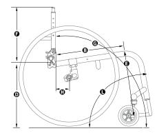
**FRONT ANGLE**  Measure from frame front to floor.
