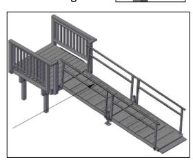
4. Install second self-tapping screw into the opposite side of each connection sleeve. Use predrilled hole in upper tube of handrail. Each rail joint should have one connection sleeve and two screws.
