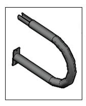
4. Finish installation by sliding the exposed connection sleeve into ramp handrail. While holding the joint tight, install provided self-tapping screw through predrilled hole in the upper rail. With the upper connection completed, secure handrail starter bracket into handrail with 2 self-tapping screws. Install remaining screws to complete the connection.
