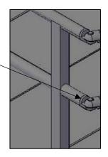
3. Slide another elbow (#3) into upper ramp handrail but do not secure with screw yet. For lower handrail, you will first need to install a handrail starter bracket before sliding in the adjustable elbow (#4). The height of the handrail starter bracket should be matched to that of the other lower rails.
