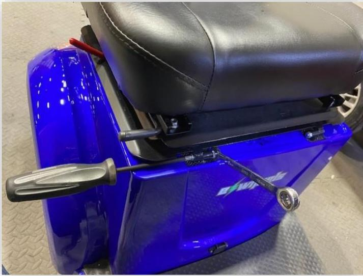
The seat is secured by two bolts, and the seat latch. The seat bolts are a 5mm hex head bolt on the bolt side, and 10mm on the nut side. Avoid overtightening or the seat will not be able to be lifted easily.
