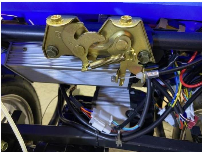
Remove the cable that goes to the truck lock. Your going to want to pull up in the meal/plastic part and remove the end of the cable.
