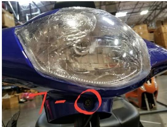
**Key Note -** The speedometer can be removed as well if needed once this has been completed. A 10mm socket and ratchet can also be used to remove the outside bolt.
