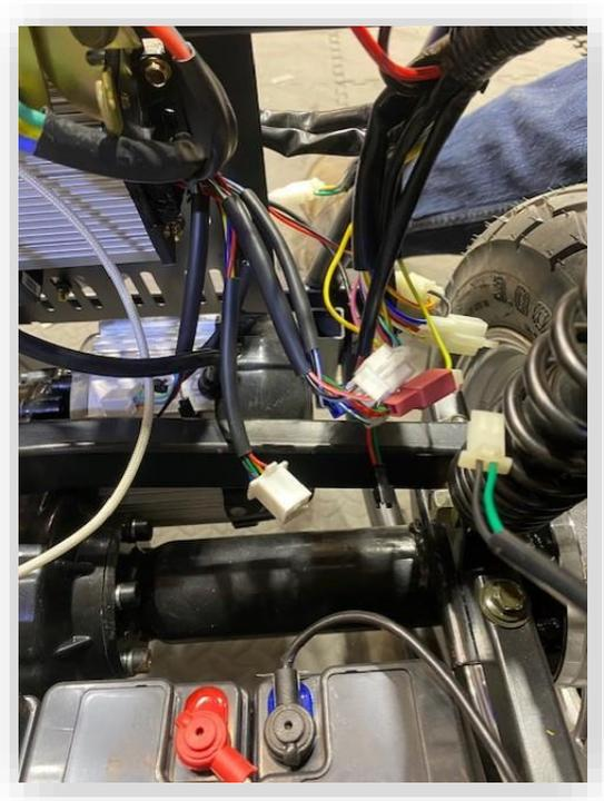
Once all connections have been replaced, remove the old wire harness and the entirety its mounts. Zip tie the new harness to the frame at the same points the old harness was mounted. Test that all functions of the scooter are working as they should prior to reinstalling the body paneling.
