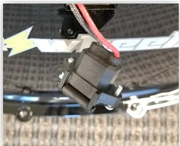
from the wire harness and install the new charger port.
