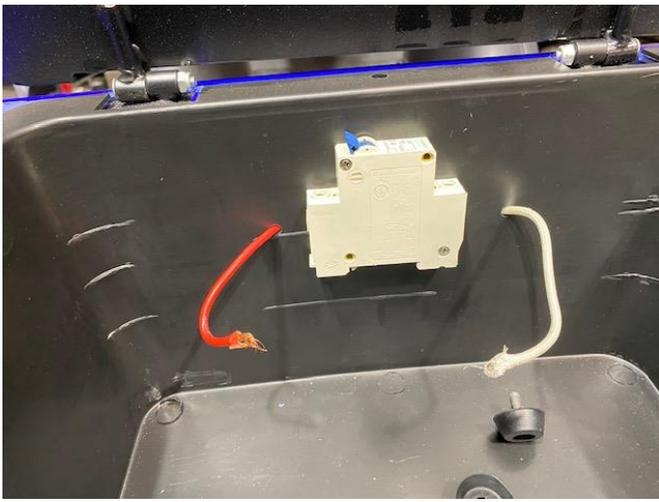
You going to want to remove both wires going to the circuit breaker before removing the storage box.
