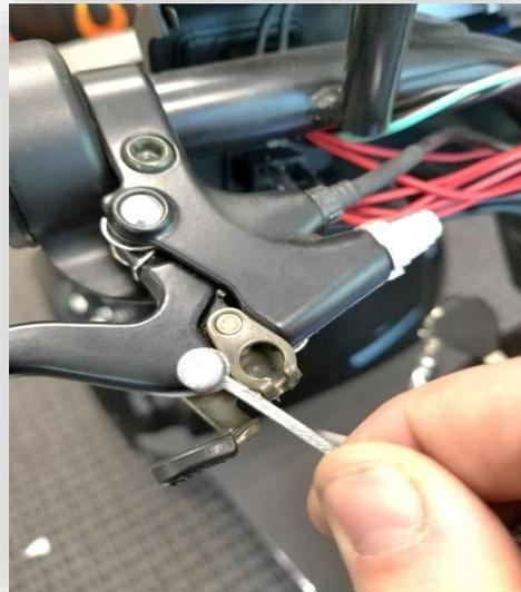
**Left Brake Handle Replacement** - To replace the left brake handle, start by removing the headlight shroud. Once removed, take off the securing nut and bolt. Both the nut and the bolt are 10MM.
