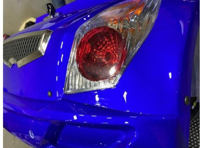
Remove the 2 screws on the edge of the main body shroud that hold on to the rear bumper. There are also 2 screws to the left and right of the chrome and black piece that need to be removed.
