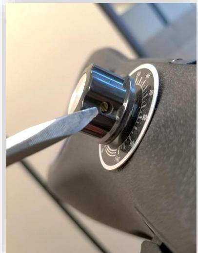
**Button Replacement** – To replace the high/low beam, turn signal, forward/reverse, or horn button, start by removing the headlight shroud. Once removed, locate the button you intend to replace, and separate the electrical connector. Then, dismount the original button by depressing the push clamps on each side of the button. A flat head screwdriver can help to depress the push tabs easier.
