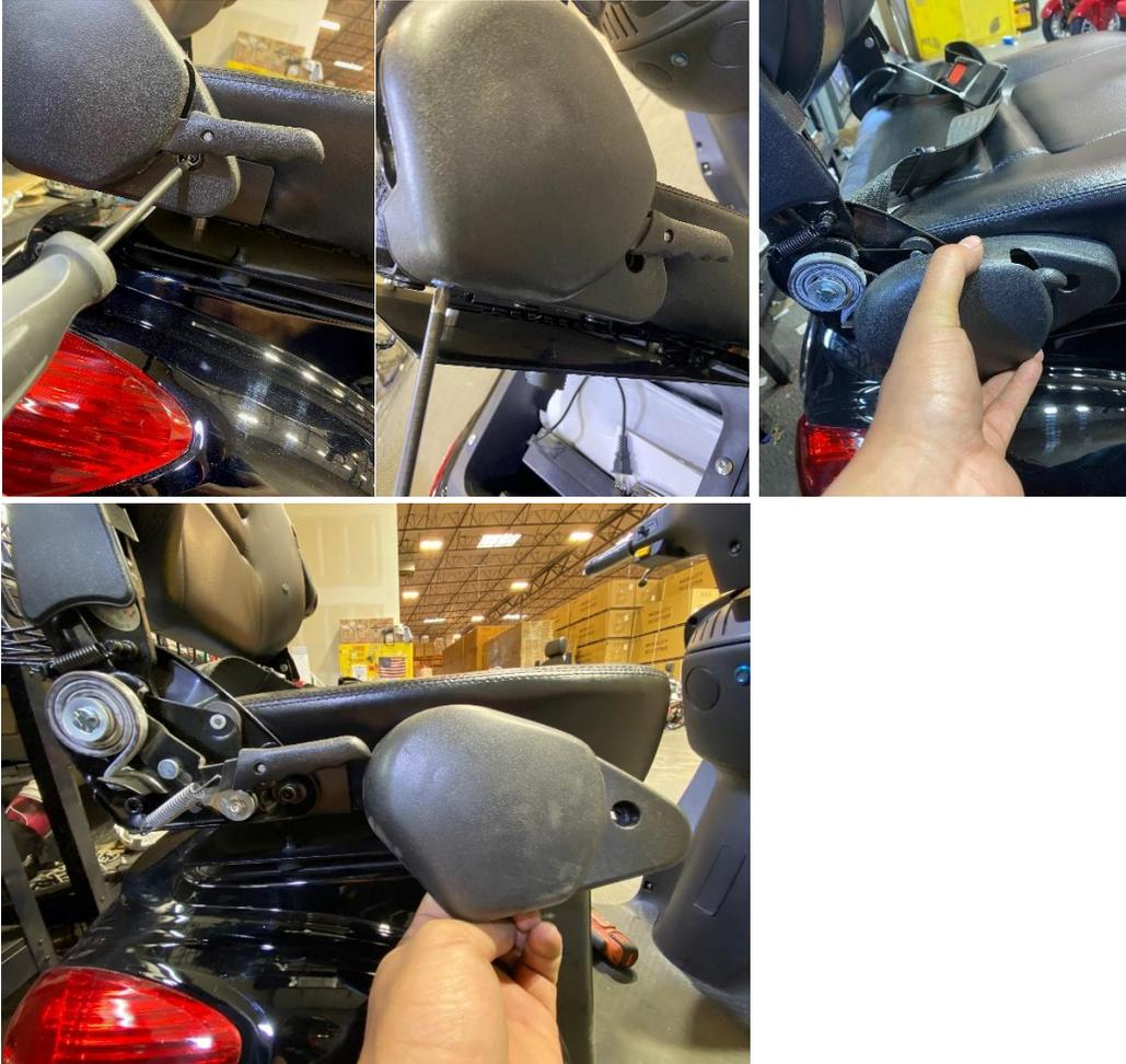
Lifting the seat up may make it easier to get to the screw on the bottom side. You will slide this plastic cover off the lever on the seat as shown in the photo.
