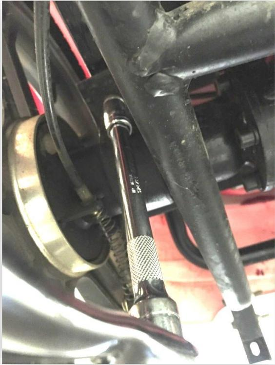
There are two transaxles to swing arm bolts on each side of the scooter. The bolt side is a **Correct Size To Use**. Make sure the bolts are tight on each side. If there is a gap between the axle bracket and the swing arm, this is normal. If overtightened bolts from the transaxle to swing arms can potentially snap.
