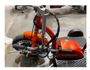
Make the handlebars and tires are aligned then carefully fold handlebars down and tight the **6mm** Allen wrench bolt. You can use your feet to hold the front wheel while doing so.
