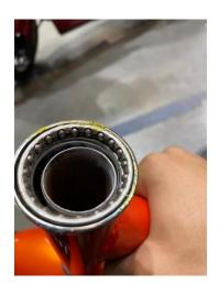
After loosening the bolt, you are going to want to remove the big nut that is holding the forks in place. Once you have removed the nut you will want to be careful pulling up the frame as the bearings might fall out.
