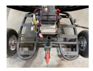
We will be removing the handlebars from the front forks also, so you are able to take the front forks off as well. Fold the handlebars down and get a **6mm** Allen wrench to loosen the bolt underneath.
