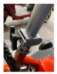
You are going to want to untwist the plastic knob until the metal part is loose enough to fold the handlebars down.
