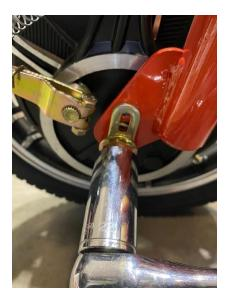
For the front tube & tire the nut will be the 22mm socket or wrench to take it off front forks. Be carful of the motor wire when doing so as well.
