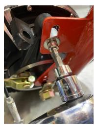
There is a 5mm Allen wrench bolt that helps hold the brake housing on that you need to remove as well.
