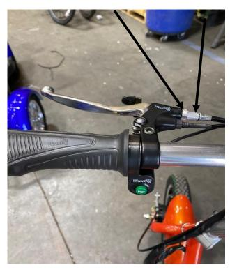
Making sure you have your parking fully released. There are 2 parts the arrows are pointing to where you can make some minimal adjustments to loosen or tighten the brake tension.
