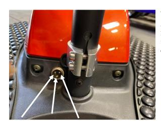
You want to set the multi meter to DC-100, put it on the prongs as shown in the photo. It should be admitting 12Volts or higher if charged (Max 38-40Volts).
