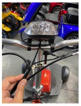
Making sure all the connections at the headset are connected and don't look pulled out. Also going in under the cover to double check battery connections and all others as well would never hurt.
