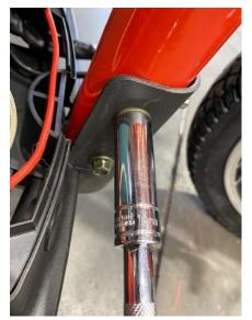
To remove the front portion of the frame you will need a **14mm** socket or wrench
