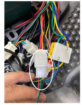
To test that the controller is emitting the proper voltage to the motor, connect your multimeter to any color combination on the motor phase wires where they connect at the yellow junction box. Set your meter at DC 50 or higher, and test under load (with the scooter power turned on, while pulling the throttle). The voltage should start at 0 and increase between 2.5-3.6 volts while under full load (holding the throttle pulled at the way).
