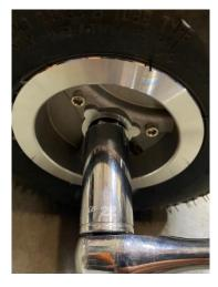
Its going to be a 22mm socket and rachet that will be used to take of both rear wheels when changing the tubes.
