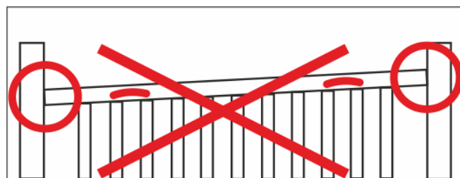
Fig. Incorrectly locked siderail
