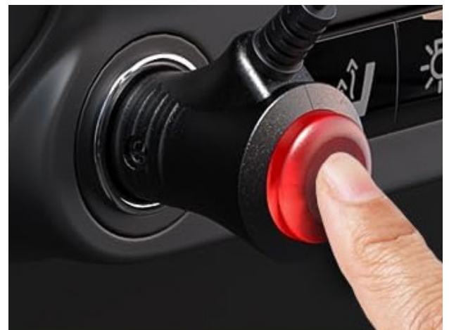
Turn monitor on/off by pressing switch on accessory port
