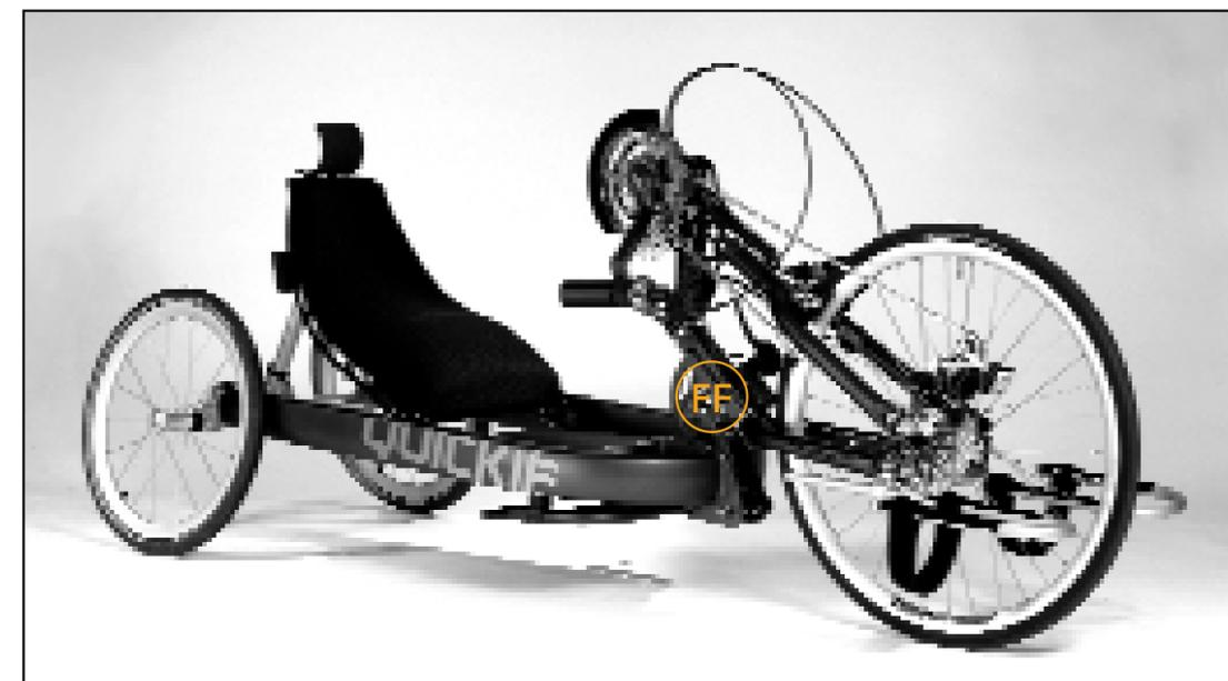
FF Frame and fork can be separated for easy transport and storing of the bike.
