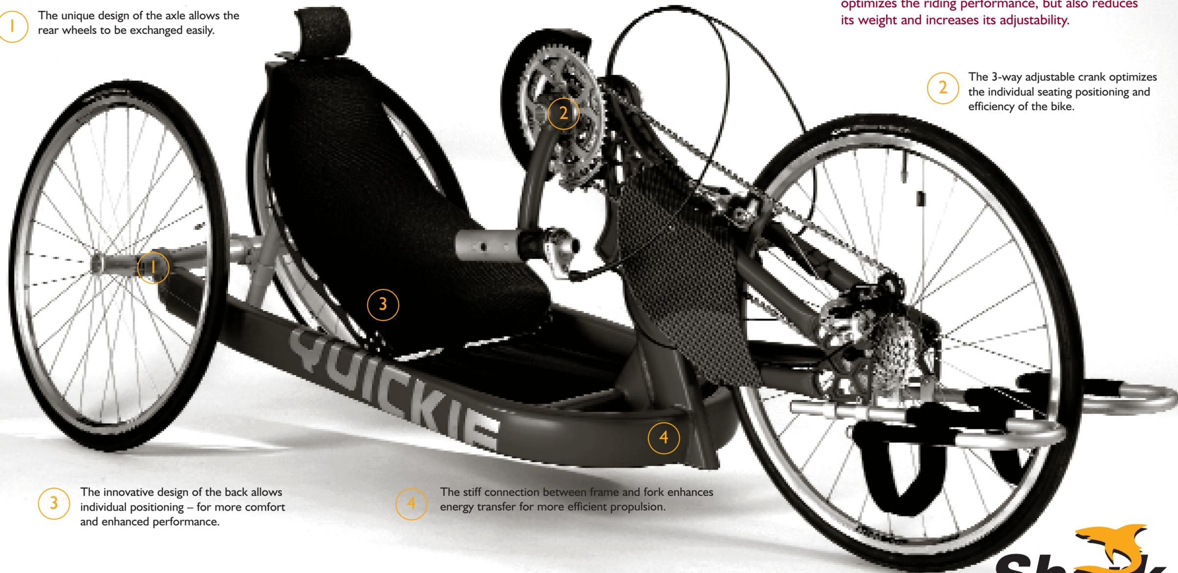
2 The 3-way adjustable crank optimizes the individual seating positioning and efficiency of the bike.
