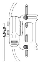
The angle and the depth of the backrest are adjusted, if needed, at the same time. Loosen the two bolts on the bracket and adjust the angle and depth of the backrest in one movement. Retighten hardware once desired configuration is achieved.
