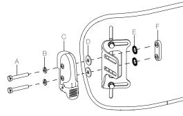
Install backrest mount clamp (B) to mount plate (C) using two lock washers (E), two spherical washers (D) and a dual nut (A). Bolts should thread inwards from the outside of the chair. Choose bolts, from the two sizes provided, that adequately thread through dual nut without coming up short or sticking out excessively. Loosely tighten hardware inward and rearward at a 45 degree angle, snugging just one bolt. Repeat with second set of backrest mount clamps.
