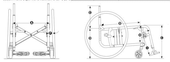
FRONT SEAT HEIGHT C Measure from floor to top of seat tube at front edge of seat sling. Adjustable in 1/2" increments. (13.5" - 14" Front Seat Height C requires Hemi Height Frame Style. 20.5" - 21.5" Front Seat Height C not available with Hemi Height Frame Style.)
