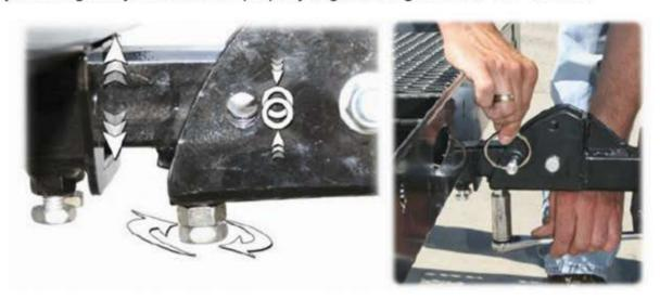
Remove Pin (17) to fold carrier vertical. Replace Pin (17) in top pin hole to secure carrier in the vertical position.
