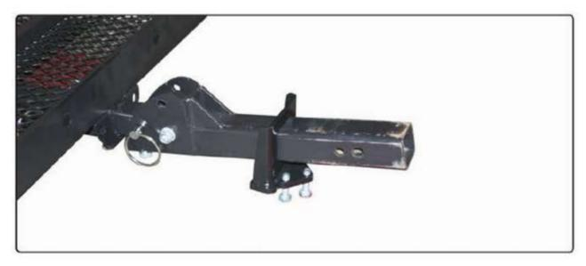
\*It is required to install either the included Anti-Tilt Locking Device (preferred) or pinch bolt (alternate option).
