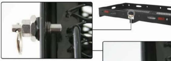
Adjust Spring Pull Pin (13) with enough room that when pulled back, the ramp (22) can be lifted out of the carrier basket (21). Securely tighten jam nut.
