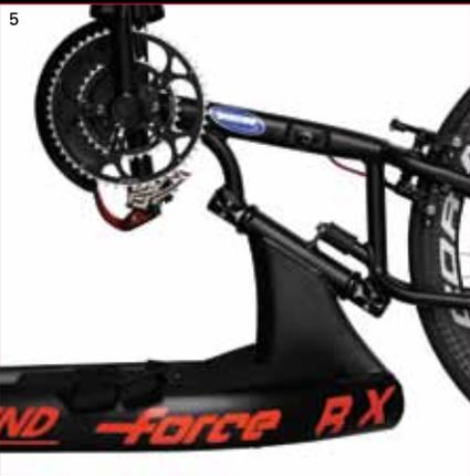
5 The redesigned curved monocoque front triangle is super strong and looks terrific. This new design allows the athlete to get closer to the front wheel which translates to a lighter and stiffer fork because it is shorter. Plus it gives the competitor more body clearance so the athlete can get lower and obtain a more streamlined position.
