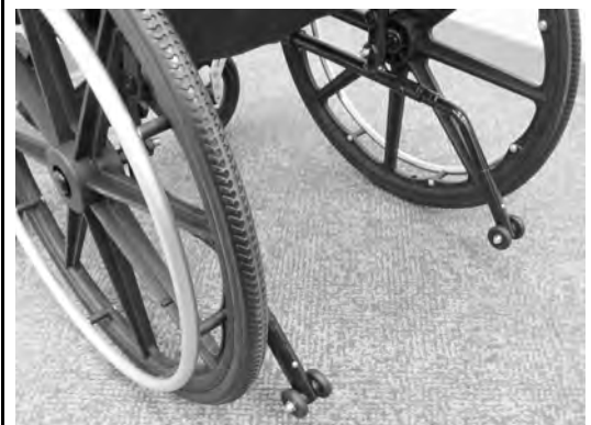
FIGURE 10.2 Changing Orientation of Anti-Tip Wheels
