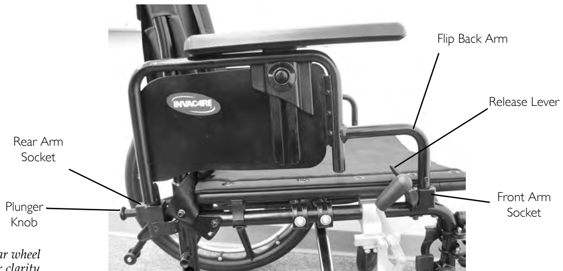
FIGURE 5.3 Removing/Installing the Flip Back Arm
