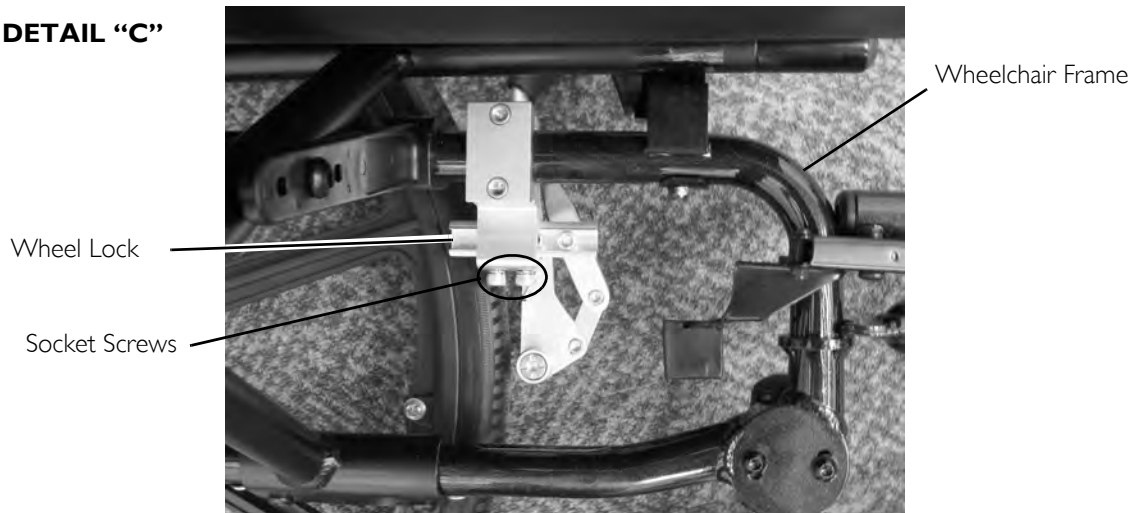
FIGURE 9.2 Adjusting Patient-Operated Wheel Locks
