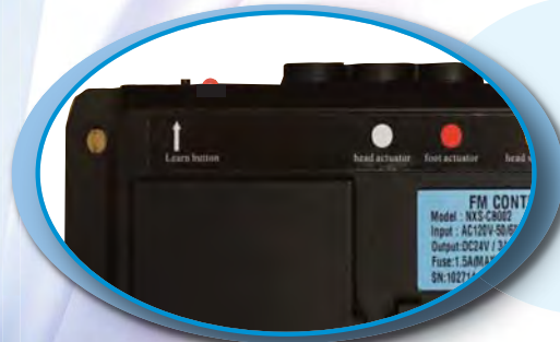
Figure 2: The red LED will light up when the control box is in the learning mode.
