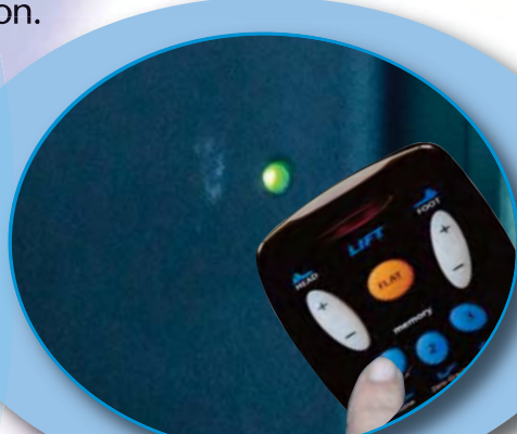
Figure 8: Lower the bed using the 9 volt battery backup system
