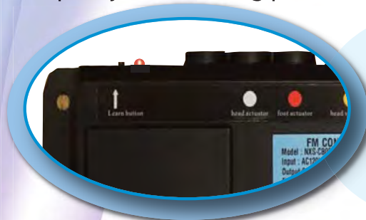
Figure 4: A flashing red LED indicates the control box has received the remote control frequency
