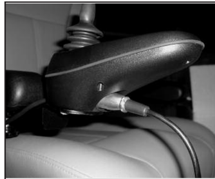
Off-board charger port (located under joystick)
