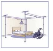
The 4 post Easytrack operates like a traditional x-y system covering all 4 corners of a room. The 4 post system is not telescopic
