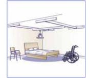
An x-y system without posts and with 4 wall brackets.
