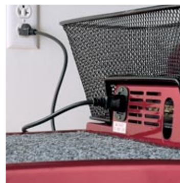
The 3-amp charger is mounted on-board to ensure that it is always available to recharge the batteries.
