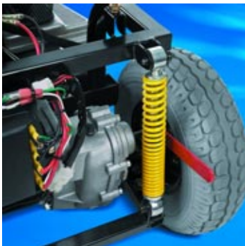
Designed with four-wheel suspension to ensure a comfortable ride.
