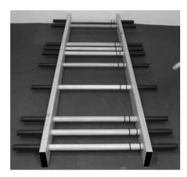
**Step 4**Lift up left rail "B" and slide the dowels in about 7".
