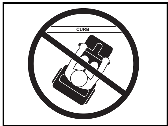
Figure 3A. Incorrect Curb Approach
