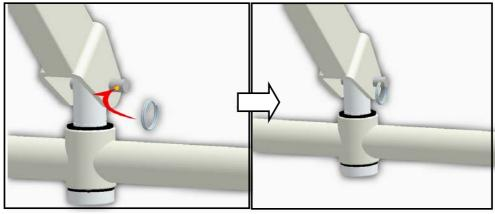
**Step 2.** Attach the Gray Control Box Hanging Bracket to the Caregiver handles on the Mast. (Notice this step is only for the Genesis 400LE)
