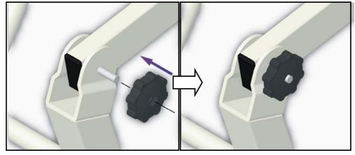
■ Secure Spreader Bar to Boom
