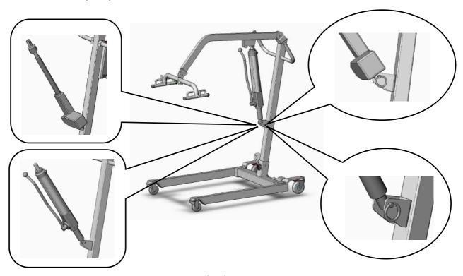
**B.** Attach the top of the Actuator to the top bracket on the Boom and insert the keeper pin and key ring.
