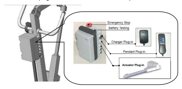
**NOTE:** Prior to using the Genesis 400LE, charge the batteries overnight. (CHARGE FOR AT LEAST 10 HOURS BUT NOT MORE THAN 12 HOURS)
