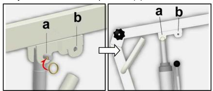
**3.** If you have an Electric Retrofit Kit, attach the top of the Electric Actuator to the Boom.
