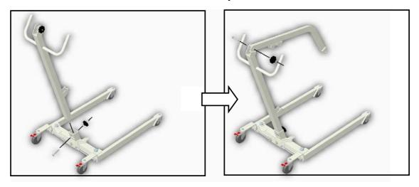
STEP 3: Pump/Actuator, and Spreader Bar
