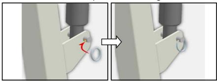
Attach the top of the Hydraulic cylinder or the electric Actuator to the Boom bracket. (See diagram below)
