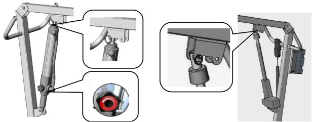
C. The Spreader Bar is attached to the Boom of the 400H /400LE by the Keeper Pin and key ring as seen below.
