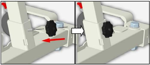
■ Boom to Mast and Tighten SECURELY.
