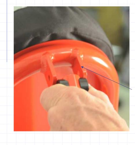
Remove bolt, nut and washer
