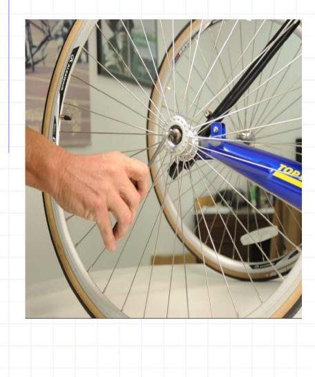
Secure each rear wheel to frame with 6 mm wrench.
