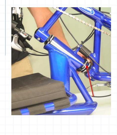
Slide lower half of clamp over lower section of the front of the frame.
