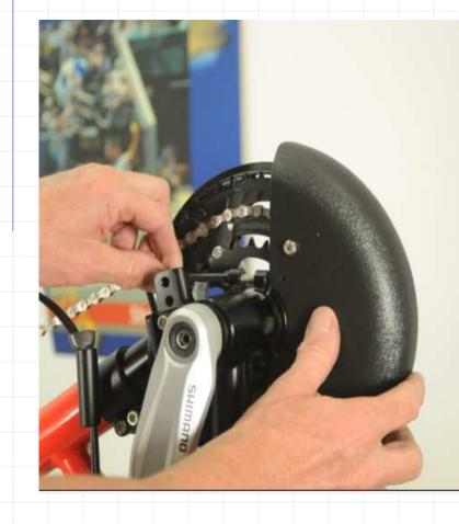
Tighten clamp assembly on left side
