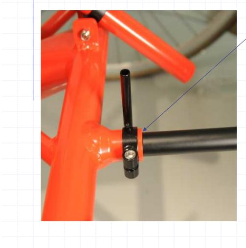
Slide flag holder over bumper receiver in the place of clamp you just removed
