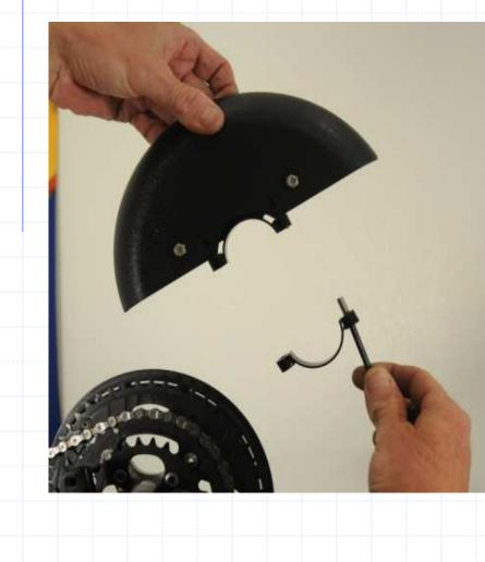
The clamp-on chain guard attaches to the crank assembly
