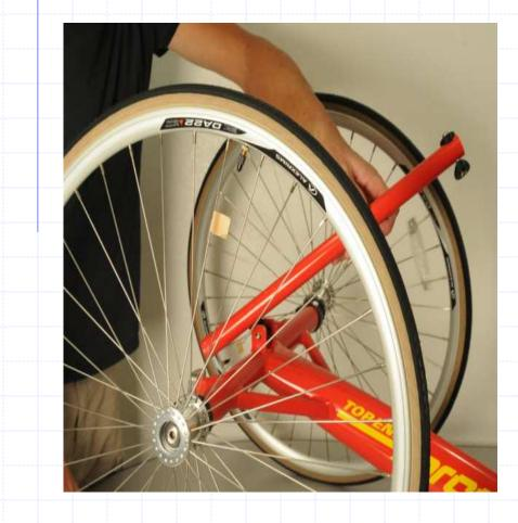
Remove backrest support bar from clamp on frame
