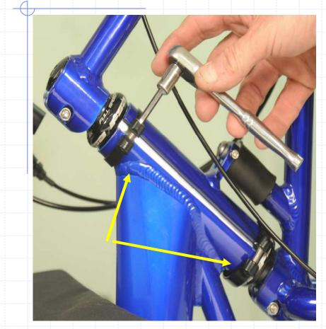
Firmly tighten both upper and lower clamps.
