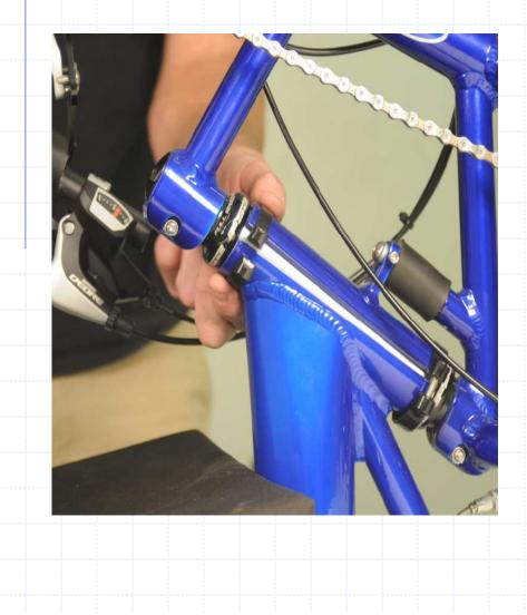
Place second clamp over the frame and the fork/frame attachment plate.
