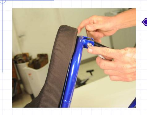
Tighten the top of backrest support bar to top of backrest using 5mm wrench and 10mm box wrench
