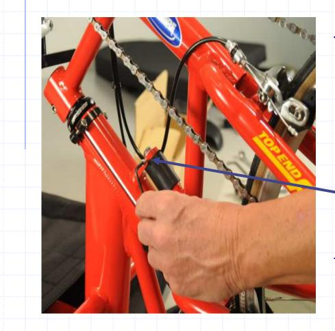
To center front wheel, with dampener bolt slightly loose, tighten set screws
