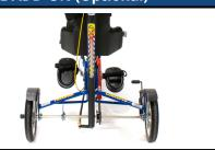
The narrow frame option has a width of 29" and is able to fit through standard door frames.
