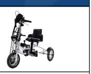
The standard EHDU12 model accommodates an arm length range of 16"-24" and an inseam range of 13"-21".
