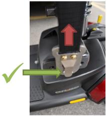
11. Engage the keyhole plates securely to the lifting bracket. (This bracket will vary depending on what is being lifted)
