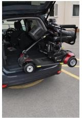
12. Press and hold up button to raise the scooter/chair up to the upmost position then release button steady the scooter during operation and ensure it does no contact the vehicle.
