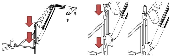
1. Rest the upper mounting lug onto the longer upper pin before aligning the lower pin. The hoist should slide smoothly down into place.
