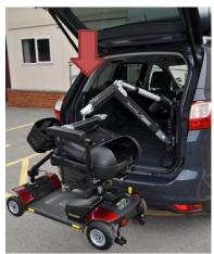
10. Press and hold the down button until the scooter/chair is grounded and there is some slack on the lifting straps.
