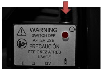
15. Press the power button (the indicator red light should no longer be illuminated indicating power OFF)
