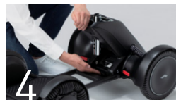
4 Pull the lever on the side of the battery toward you to separate the parts.
