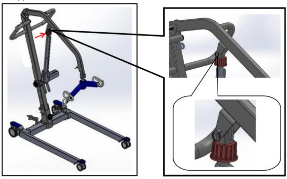
**Step 3.** Attach the Control Box to the Mast and tighten two screws.
