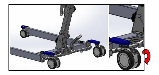
**Step 2.** A. Remove another QR pin which is connected to the bottom of Actuator and Boom. Leave the QR pin on Boom as below left picture.
