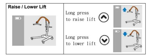
3. Press the button to raise or the button to lower the lift.
