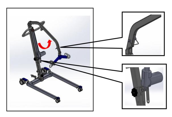
B. Attach the top of the Actuator to the bracket on the Boom and insert pin. Insert keeper ring through hole in pin to secure actuator to upper bracket.
