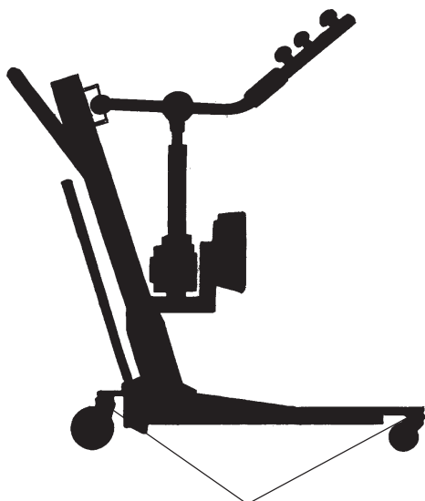
Lubricate the Bearings in the Caster Swivels
